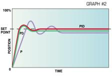
In order to decrease the error even further, a third function,"I", is added to the "PD" servo. The integrator ("I") slowly decreases the error when the position reaches stability. This addition of the "I" function converts the ICoT into a "PID" servo type system.
