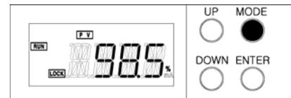
Push DOWN for more than 5 seconds, and SPAN will be displayed.
