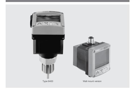
This Transmitter/Switch is specially designed to switch a valve, pump, heaters, etc... and establish an ON/OFF control loop. The switching point can be programmed with the 3 key pads on the display or externally from a programmable logic controller via a 4-20 mA loop. Additionally, the process value can be transmitted to the PLC (4-20 mA). The connection to the process in the piping is done with standard fittings.
